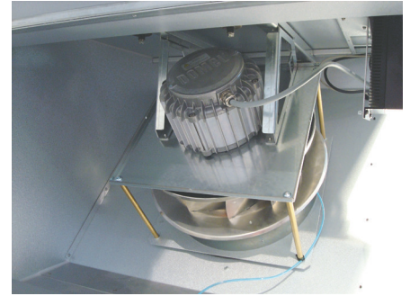
The motor sections are mounted in vibration dampers, which reduces noise in the ducts and eliminates the need to fit flexible connections between the unit and the duct system.
