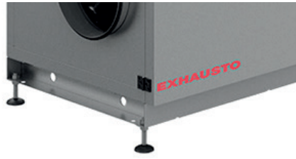
Mounting base is an accessory for VEX140-150-160 and standard on VEX170. The mounting base is equipped with feet that have an adjustable height of 130 - 160 mm.
